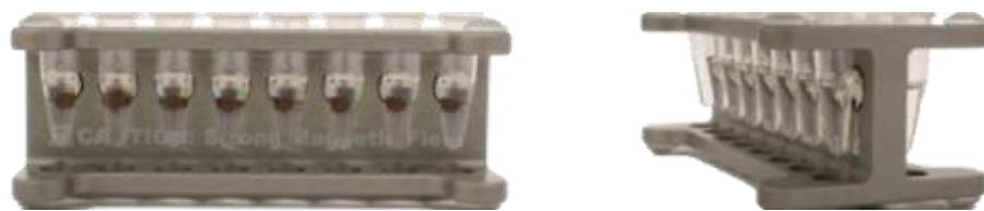
Figure 2: Clear supernatant with compact bead pellets.
