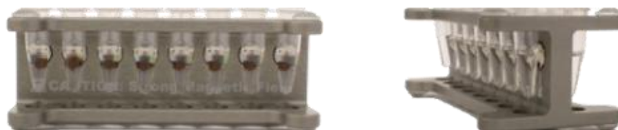
Figure 2: Clear supernatant with compact bead pellets.
