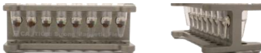
Figure 6: Clear supernatant with compact bead pellets.
