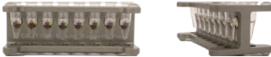
Figure 4: Clear supernatant with compact bead pellets.
