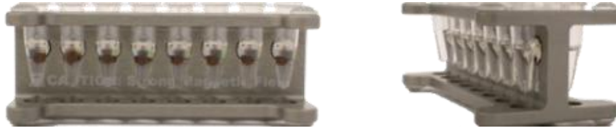
Figure 4: Clear supernatant with compact bead pellets.
