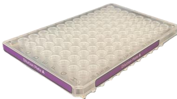
Figure 3: Image of sticker placement on a Semi-Skirted 96 Well PCR Plate. Place one sticker on the left side of the plate, adjacent to column 1, and the other sticker along the bottom edge, next to row H. This reduces contact with the plate seal.
