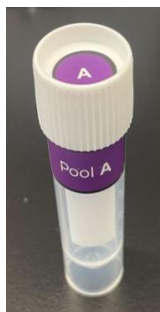
Figure 7: Ensure the stickers on the side of the tube are as close to the top of the tube as possible to ensure the 5mL tube fits correctly in the Parse Metal Cold Block.
