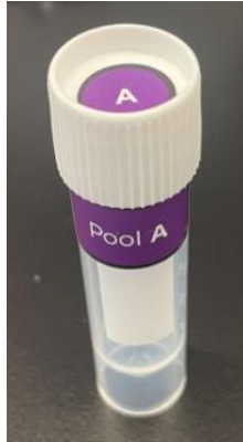
Figure 7: Ensure the stickers on the side of the tube are as close to the top of the tube as possible to ensure the 5 mL tube fits correctly in the Parse Metal Cold Block.
