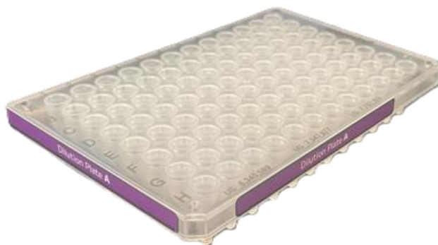
Figure 3: Image of sticker placement on a Semi-Skirted 96 Well PCR Plate. Place one sticker on the left side of the plate, adjacent to column 1, and the other sticker along the bottom edge, next to row H. This reduces contact with the plate seal.
