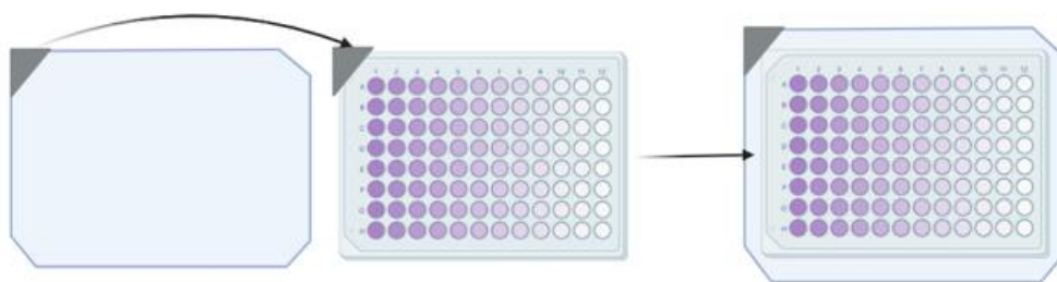
Figure 7: Corners are aligned between the Thermochromic PCR Cold Block and the Thermochromic PCR Cold Block Riser.
