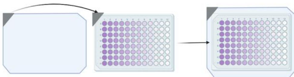
Figure 7: Corners are aligned between the Thermochromic PCR Cold Block and the Thermochromic PCR Cold Block Riser.
