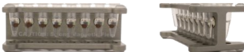
Figure 3: Clear supernatant with compact bead pellets.
